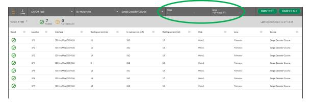
Results are displayed in a table showing the different current values at each step (Resting, In-Rush and Holding).
