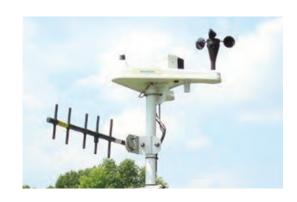
equipment, it needs maintenance. Lack of maintenance over the years can cause your weather station to not provide the correct data. Often times, weather stations are then unplugged from the system, causing your central control system to be less efficient leading to over or under irrigating.
