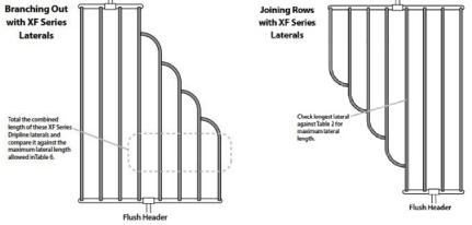
When joining lateral rows from a supply header, check only the longest lateral against the maximum lateral run length listed in Table 6 (pg. 21) in the guide.
