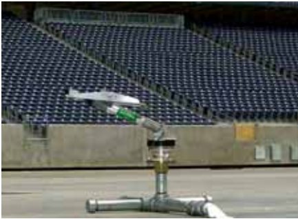
To feed water to the Rain Guns, a 2" fire hose is used. The use of cam lock couplers simplifies the connection process, and each sprinkler has its own control valve to allow the grounds personnel flexibility in watering the turf.
