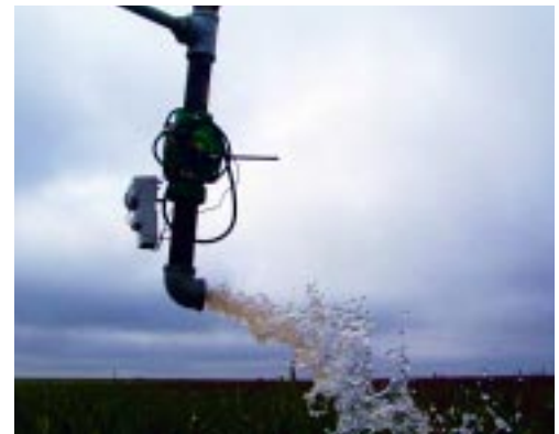
The valve opens for 40 seconds every 3 hours to flush sand.
