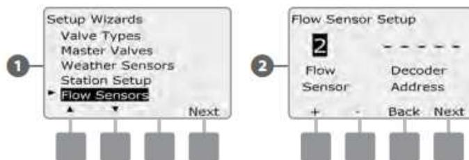
2. Press the + and – buttons to enter the decoder address; then press Next.
