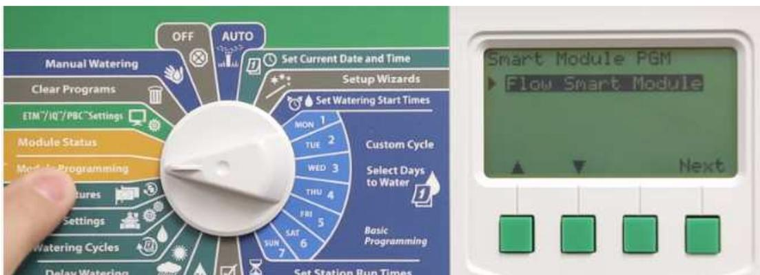
Using the up and down buttons select Set Flow Rates; then press next.
