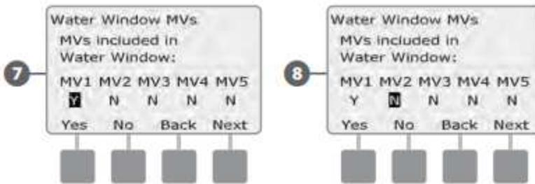
9. If FloWatch is enabled, the controller will request incremental flow allowed for the MV Water Window. Press the + and – buttons to enter a sufficiently large value so that flow from hoses and other manual watering devices will not trigger a false SEEF alarm.
