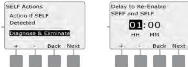
Press the + and – buttons to set minutes before Re-Enable; then press Next.
