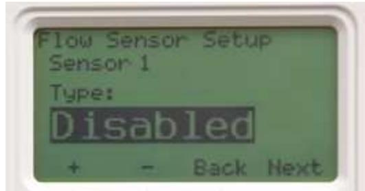
4. Press the + and – buttons to select the Sensor Model. In our example we will select the FS150P; then press Next.
