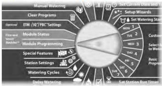
1. The Smart Module PGM screen appears with Flow Smart Module selected; press next.
