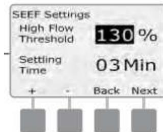
Settling Time is selected, allowing you to set the minimum time (from 1-10 minutes) that a flow rate must remain at (or above) the threshold before the controller will issue an alarm or take action. Rain Bird recommends 3 minutes. Press the + and – buttons to set the Settling Time; then press Next
