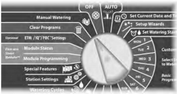
1. The Manual Watering screen appears. Press the Down Arrow button to select MV Water Window; then press Next.
