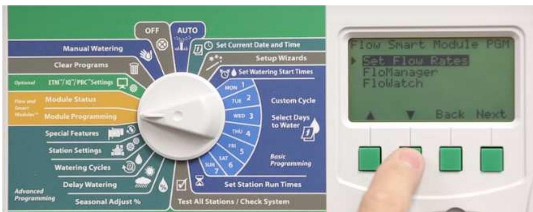
Select the Learn Flow with up and down buttons; then press next. Rain Bird recommends this method. We do not recommend setting the Station rates as this may not be accurate.
