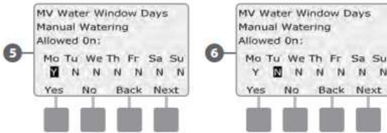
7. The MVs included in Water Window screen appears allowing you to choose which MVs to include in the MV Water Window. Press the Yes button to include the selected MV in the Water Window or press No to exclude it.
