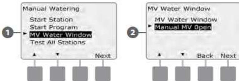
3. The Manual MV Open screen appears, showing all MVs that were previously selected to be included in the MV Water Window; press Next
