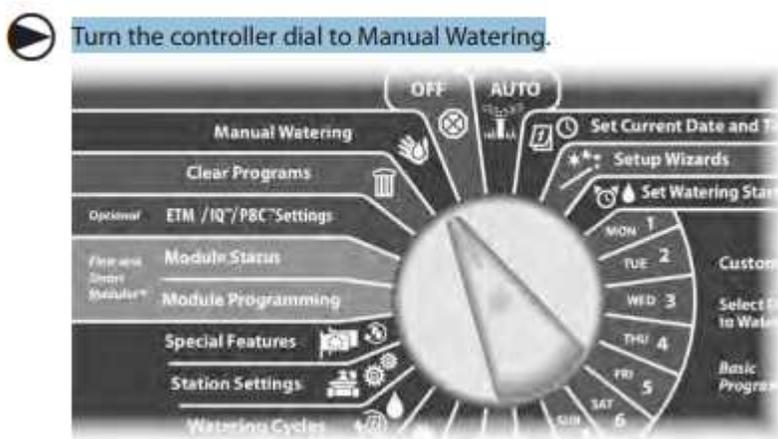
1. The Manual Watering screen appears. Press the Down Arrow button to select MV Water Window ; then press Next.
