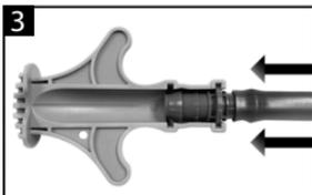
Once the end of the dripline has been flared, push dripline onto fitting.
