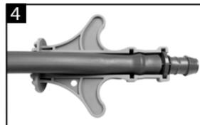
To insert dripline on the other end of a fitting, turn the tool around and lock fitting with dripline into place. Then, repeat step 3.
