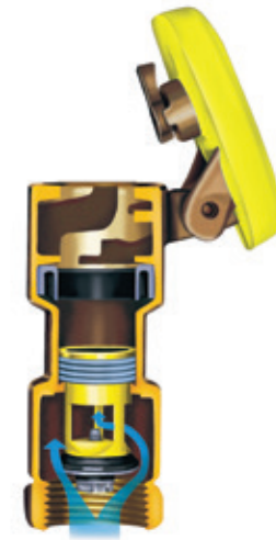
Quick-Coupling Valve Cutaway
