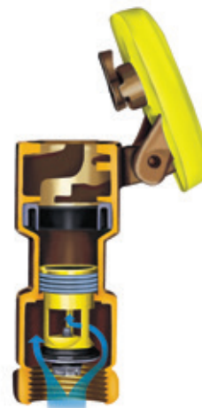
Quick-Coupling Valve Cutaway
