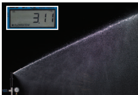
5000 PRS Rotor with 3 gpm nozzle at 79 psi inlet pressure. PRS regulated flow to 3.11 gallons per minute.
