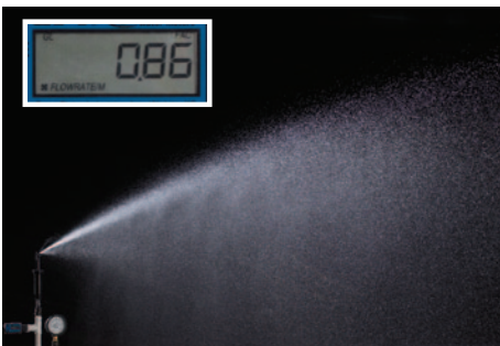
1800 PRS Spray with 15Q nozzle at 79 psi inlet pressure. PRS regulated flow to 0.86 gallons per minute.
