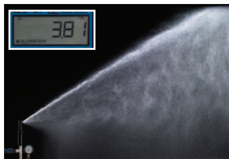
Non-PRS competitive rotor with 3 gpm nozzle at 79 psi inlet pressure. Without PRS, flow rose to 3.81 gallons per minute.
