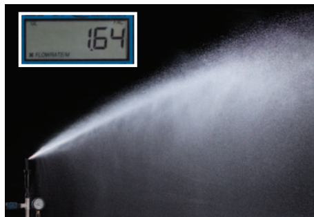
Non-PRS competitive spray with 15Q nozzle at 79 psi inlet pressure. Without PRS, flow rose to 1.64 gallons per minute.
