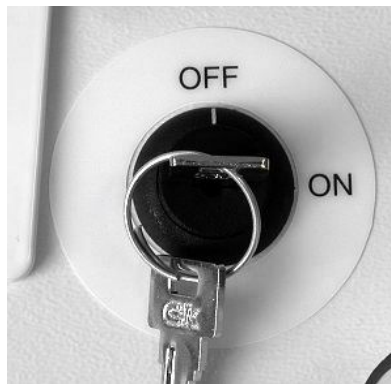
FIGURE 4-3. Keyed power switch is located on the bottom of the WS-PRO LT
