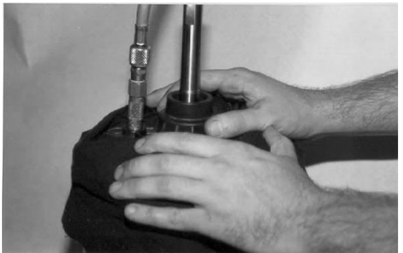
Figure X-2 Hook air to motor base plate, firmly grasp motor base plate with two hands and pressurize to 5 PSI. Note: wrap a shop rag around motor base plate seat to catch residual oil that may escape as the assembly pops open.
