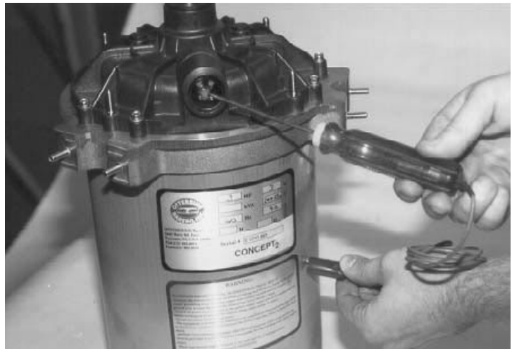
Figure X-27 Continuity check to S/S housing.
