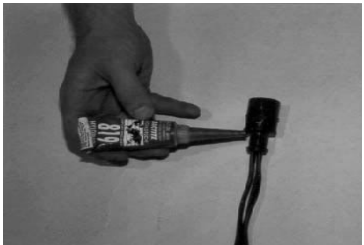
Figure X-11 Apply gasket dressing to bulkhead insert as shown.
