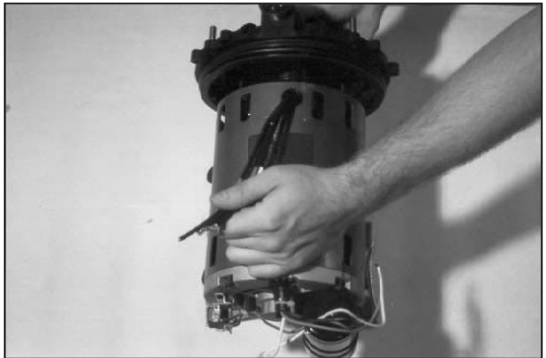
Figure X-19 LM motor/motor base plate pre-assembly.
