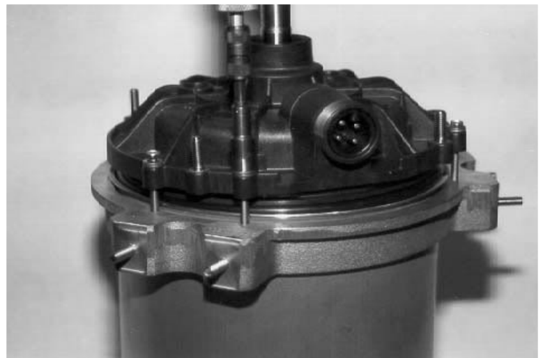
Figure X-26 Insert the (6) bolts and (12) washers into the motor base plate at the proper locations.
