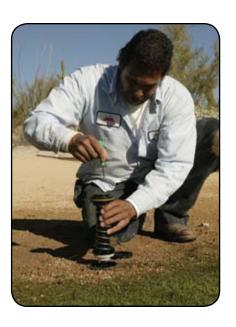
The EAGLE 351B is fully top serviceable—no need for digging. Available with NPT, BSP, and ACME inlet threading, the EAGLE 351B block rotor is ready for immediate installation in your golf course. Select the nozzle that's right for the job and you're ready to irrigate to incredibly specific distances and locations. For part- or full-circle operation, simply turn the selector to the desired setting—you won't need to change the whole internal assembly.
