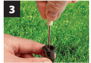
3 Distance Adjustment Turn screw clockwise to reduce up to 25%.
