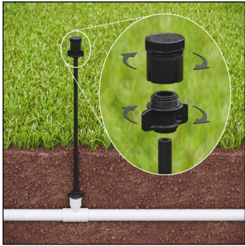
SQ Nozzle on PolyFlex Riser Assembly (PFR-FRA)
