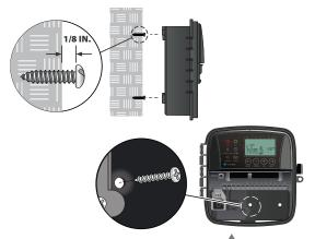
If hard wiring for AC power, remove knockout for conduit
