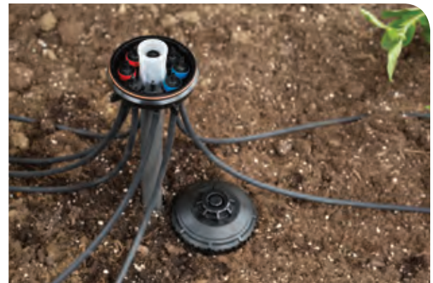
Each port can be configured on the Xeri-Bird™ by installing flow controlled emitters. Above shows a combination of 0.5, 1.0, and 2.0 gph Xeri-Bug emitters.
