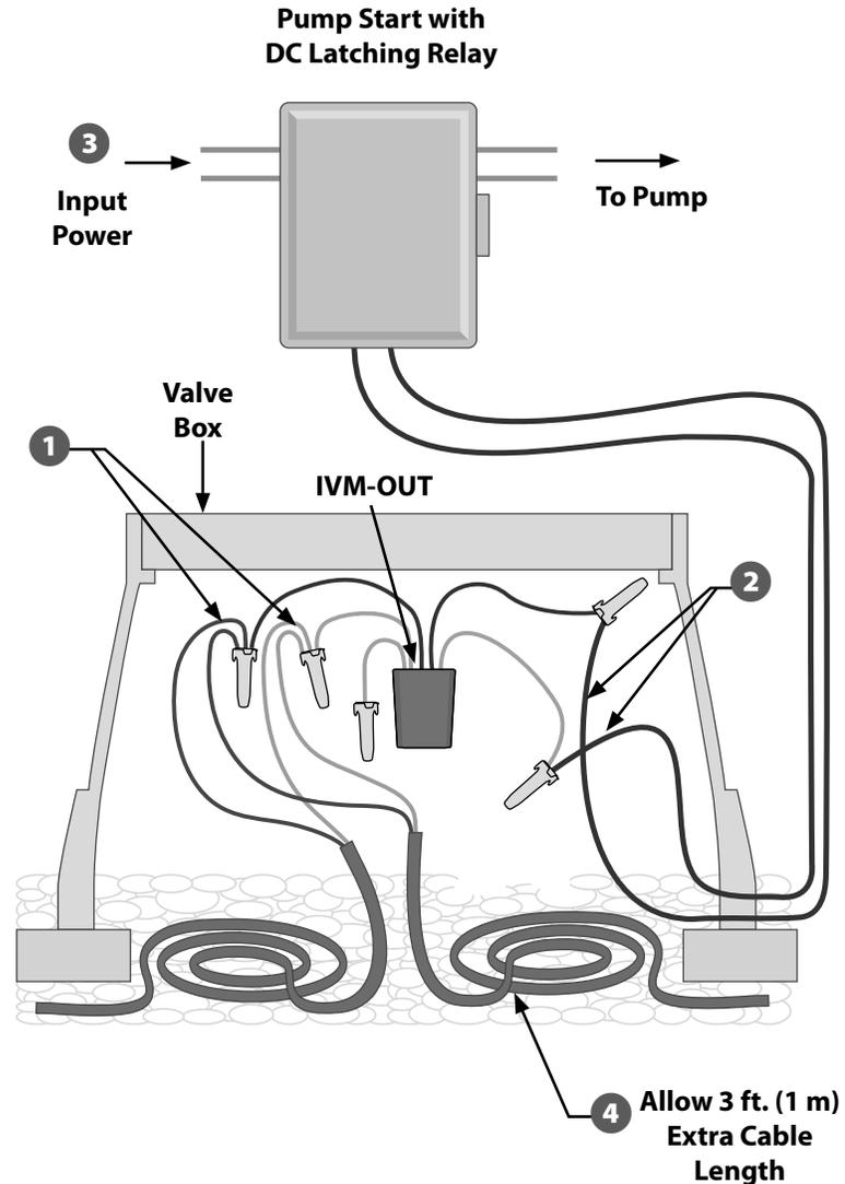
Typical IVM-OUT Pump Start Relay Wiring
