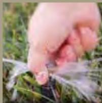
Pull up nozzle cap to flush debris
