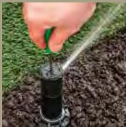
Radius adjustment screw allows up to 25% reduction of throw distance without changing nozzles.
