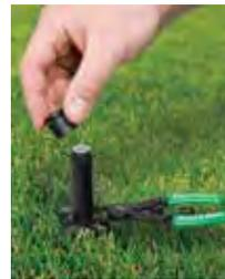
**4** Pull up stem and remove nozzle. Rain Bird Stem Pull-Up Tool PTC-1 shown (page 50).
