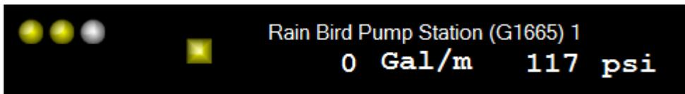
Up to 10 pump status LEDs with identical color definitions will be displayed to the left (round LEDs in 2 rows, if needed). Pressure maintenance pump and jockey pump status will be displayed to the middle (square LEDs). Station flow rate and pressure are also displayed. Other status indicators visible in the Pump Manager 2 main window are not visible. If multiple pump stations are configured, status information is visible for each as shown below:
