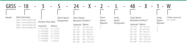
In the example above, the order is for 18 mm Heavywall Dripline with 0.53 gph emitters that features "Smart Spacing". There is a repeating pattern of 2 short spaces with emitters spaced 24" apart followed by 1 long space of 48".
