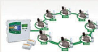
Your ESP-LXD controller is linked to decoders in the field by a two-wire path. This path carries voltage and information.
