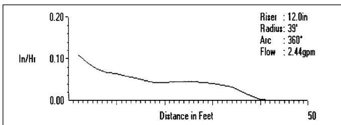
This test is conducted under zero wind conditions in a laboratory where the test pressure and riser height are fixed. Many tests have been conducted at independent facilities such as CIT in the U.S., CEMAGREF in France, and AITC in Australia. Rain Bird has conducted distribution tests at their own zero wind facility since 1980.
