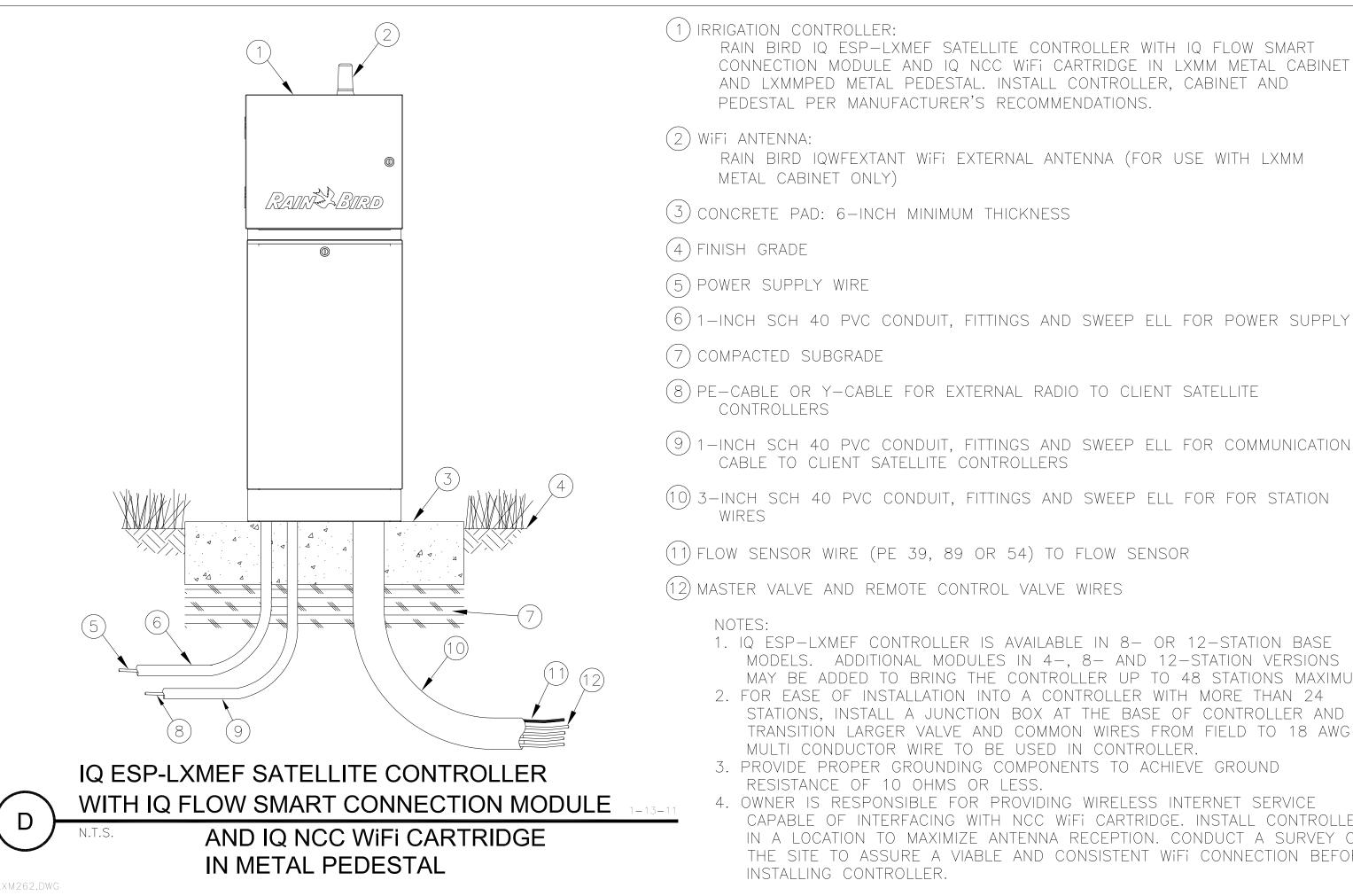
CONNECTION MODULE AND IQ NCC WIFI CARTRIDGE IN LXMM METAL CABINET
