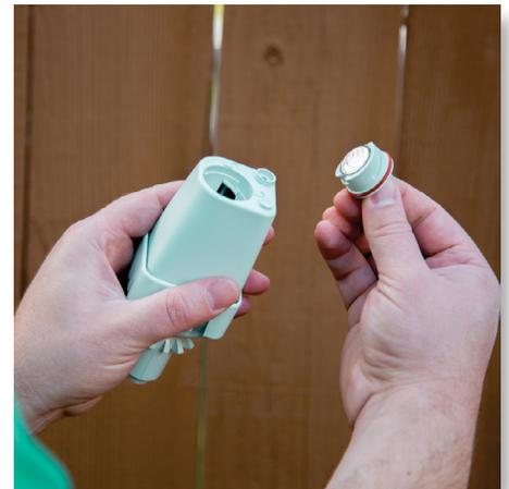
Battery replacement requires no tools or sensor disassembly
