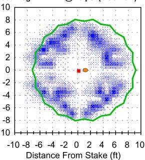
In each Treegram the blue dots represent the water pattern relative intensity. The green circular lines represent the tree canopy outline and the tree trunk is depicted by the small brown circles. The red square is the stake and is positioned in the middle of each Treegram at the origin. The "Offset Position" given in each example is the distance the stake is placed from the tree to the right.
