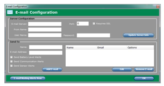
Soil Manager uses the information entered to send event emails. For example, Soil Manager could send an email when soil temperature is out-of-range, giving notification that a short irrigation to lower the temperature is needed. E-mail process configuration is split into 2 pieces: e-mail server and account configuration, and distribution list configuration including events sent to each member.
