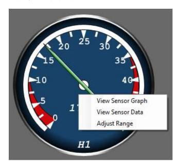
Select View Sensor Graph to open the Sensor Graph View tab and automatically graph today's data from all sensors represented by the meter (see Section 5 – Sensor Graph View). Select View Sensor Data to open the Sensor Data View tab and display a spreadsheet showing today's data from each sensor represented by the meter (see Section 6 – Sensor Data View).
