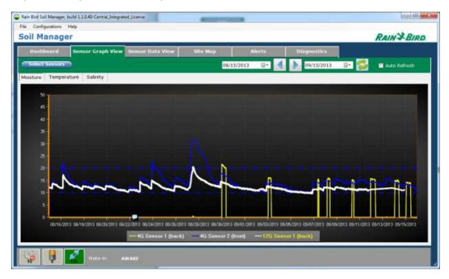
The graph view can display up to 14 sensors at a time. Additional options will be shown if 1 sensor only is selected. Those options will be discussed in Section 9 – Controlling Irrigation with Soil Moisture Data. The list of displayed sensors is set by clicking the Select Sensors button:
