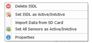
Delete ISDL permanently removes the data logger from the database, from the tree view, from the site map and no longer notes missing communication from the device as an error. If the device still exists on the network it will likely be rediscovered during the next network operation but map location and notes will be lost. To actually remove the data logger permanently (preventing rediscovery), first turn the device OFF in the field, and then delete it from Soil Manager.
