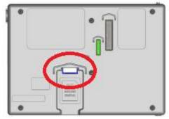
To eject the card, push the card upward a short distance until it stops and release.
