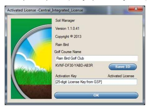
The title of the dialog will vary with the installed license type. The sample above shows a Rain Bird central control integrated license (allowing irrigation program control based on soil conditions). The Version string indicates the Soil Manager version and will vary. When requesting support for Soil Manager from your local Rain Bird office or Rain Bird GSP, **always** forward this information. The Golf Course Name can be changed to help identify the location of the PC.
