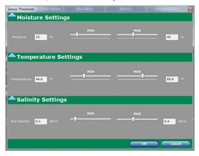
Sensor thresholds are used to detect and report field conditions requiring actions to maintain the plant material. Sensor alerts are generated in the Alerts tab (see 8.1 Sensor Data Limit Alerts for details), and out-of-range sensor values can send email notifications as well.
