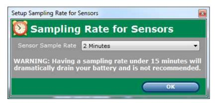
The sensor sampling rate is the frequency at which the wireless network awakens and ISDL data logger data is transmitted for each sensor to Soil Manager. Frequent sampling is desirable for short-term trend monitoring (and necessary for a time while configuring central control integration), but can drain batteries quickly. The recommended Sensor Sample Rate for stable systems is 15-20 minutes.
