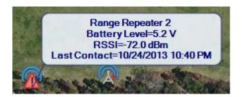
In the example above, the repeater has not been contacted recently, possibly due to bad batteries or radio issues. However, the last battery voltage received from the repeater was relatively good, 5.2V. This suggests that antenna problems, new tree or shrub growth, or other line-of-sight issues have caused the problem.
