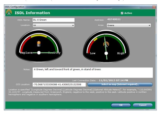
The ISDL Name is user-entered. Above a name of DL-4 Green has been entered to identify the data logger. The Address field contains the factory-assigned data logger address. When a new ISDL Data Logger is found on the wireless network a default Name value will be created based on the Address.
