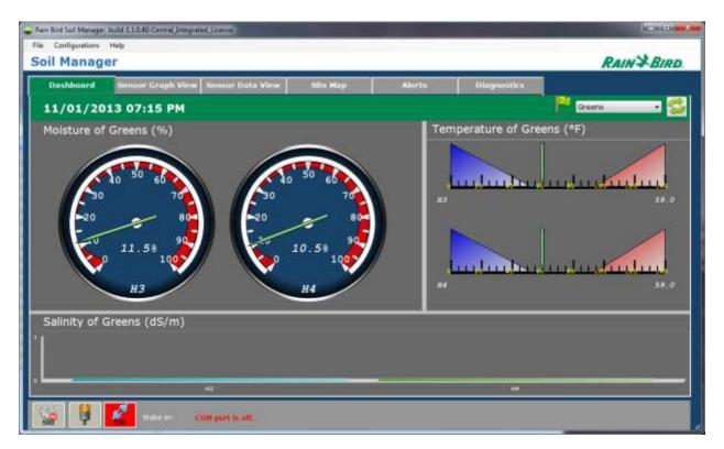
As shown holes 3 and 4 contain sensors (note 2 gauges marked H3 and H4). The sublocation "Greens" is currently active and can be changed using the pull-down list:
