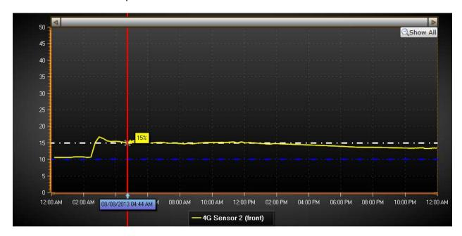
The chart display can now be zoomed to isolate the irrigation event data. To zoom, click in the graph display away from the cursor and drag to select the section of the graph including the flat area before irrigation and the peak when irrigation was completed:
