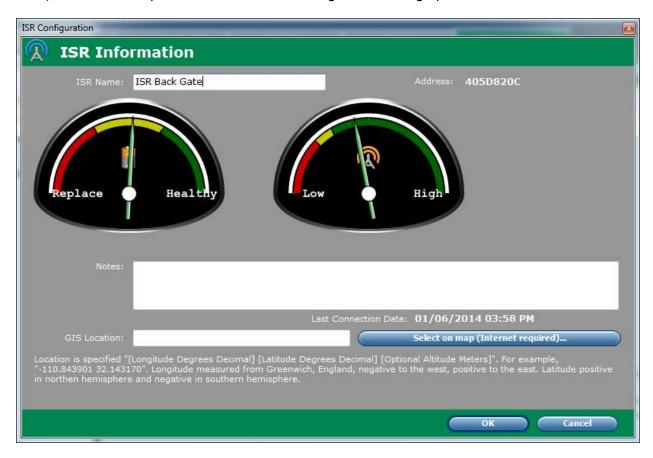
The ISR Name is user-entered identifying the location or function of the data repeater. Above, a descriptive value "ISR Back Gate" has been used. The Address field contains the factory-assigned repeater address. When a new ISR Data Repeater is found on the wireless network a default Name value will be created based on the Address.
