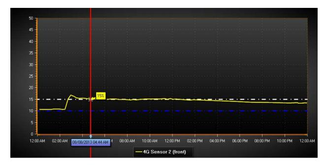
Various curve shapes may be seen. As mentioned above, a sharp peak indicates that field capacity was not reached during the event:
