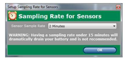
Click OK. To assure that all network devices are set for the new sampling rate, click the Sync button on the Diagnostics tab as shown below:
