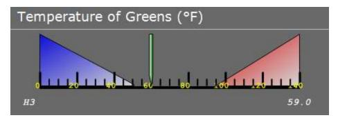
The H3 notation to the left of the graphic indicates the area location. The value to the right of the graphic indicates the average value. Note the temperature units in the title area, "°F". The units can be changed through the Unit Measurements dialog. See 2.2.1 Unit Measurements for details. The colored ranges represent the sensor thresholds set for temperature data alerts (see 2.2.3 Sensor Thresholds).
