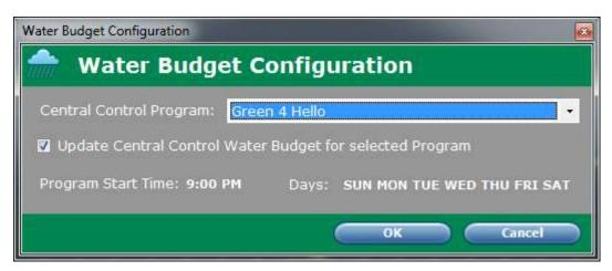
Above, the central control program called Green 4 Hello has been chosen as the calibrated program. To automatically update the central control database water budget for this program, set the checkbox Update Central Control Water Budget for selected Program. If this checkbox is unset, water budget will be calculated and displayed on the Sensor Graph View
