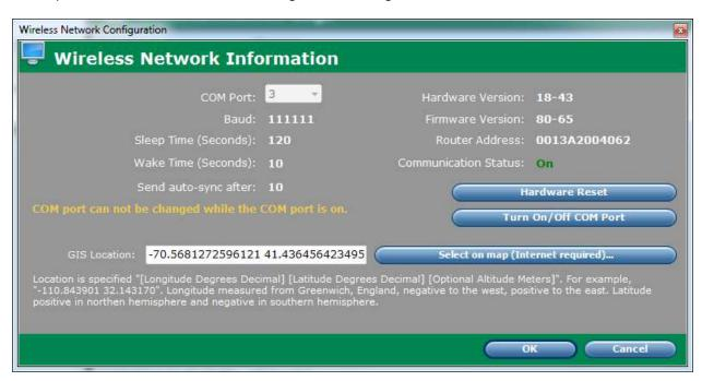
COM Port controls the serial port number through which the PC communicates with the wireless network gateway device. The value can be changed using the pull-down list, but only when the COM port is in the OFF state.
