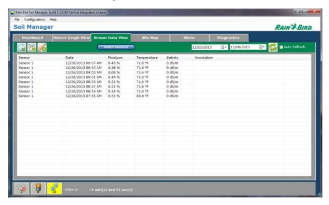
The Sensor Data View can be configured to display up to 14 sensors and many days' data. The list of displayed sensors is selected by clicking Select Sensors button shown below:
