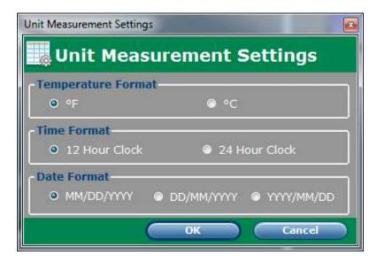
Temperature Format controls all temperature display in Soil Manager with only the exception of Communication Logs on the Diagnostic tab (see 4.2 Communication Logs) where Celcius is always used.
