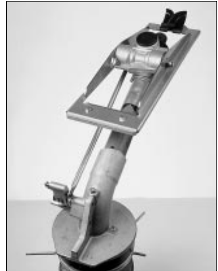
Stainless steel arm with Delrin® spoon
