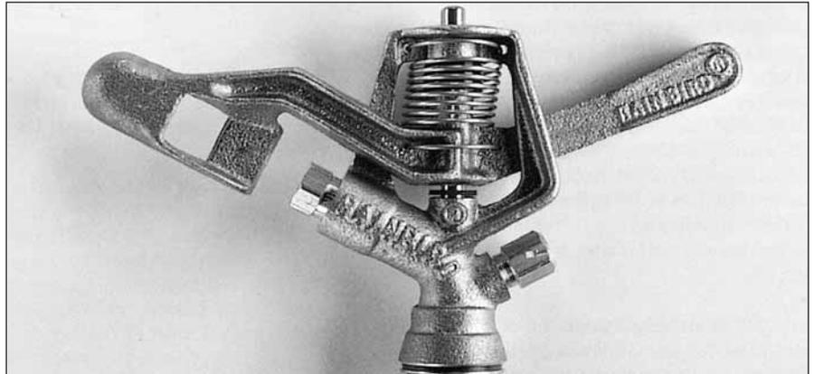
This impact is only sufficient to cause a small degree of travel so that the rotation of sprinkler is uniform and relatively slow (one-half to three minutes per revolution, depending on pressure and size of sprinkler and nozzle). Slow rotation keeps wear on moving parts at a minimum and prolongs the life of the sprinkler.
